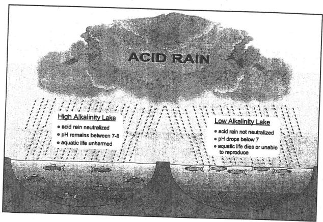
Alkalinity should not be confused with pH. The pH of a solution is a measure of the concentration of acid, or H<sup>+</sup> ions, in the water. Alkalinity is a measure of the water's capacity to neutralize an acid, or H<sup>+</sup> ions, thereby keeping the pH at a fairly constant level.
